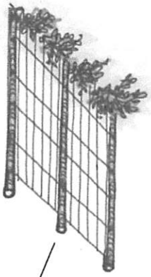
Chicken wire or hardware cloth supported by rebar
